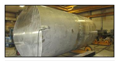
**PICTURED:** The custom-built 17,500-litre fish transport tanks to move fish from the concrete fish ladder to French Bar Creek.
